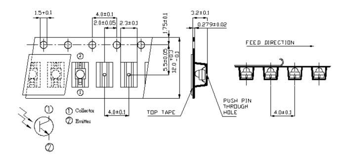
**Note:** The tolerances unless mentioned are  $\pm 0.1$ , unit=mm
