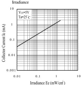
Fig.3 Collector Current vs.
